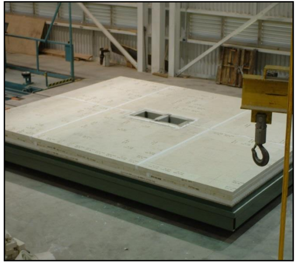
16' x 18' kiln car for 1610°C - as assembled
