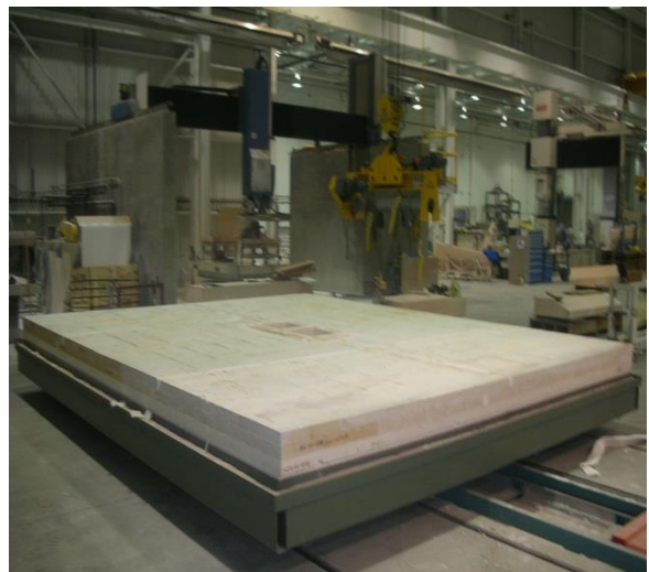
16' x 18' kiln car for 1610°C - after 1 year service
