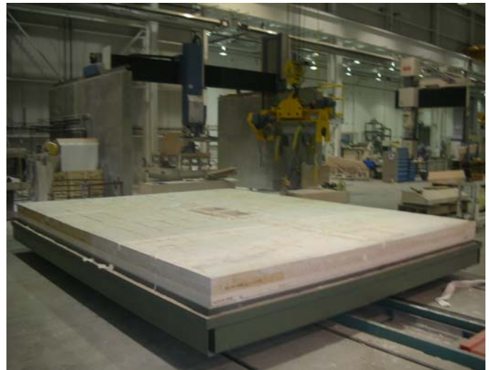
16' x 18' kiln car for 1610°C – after 1 year service
